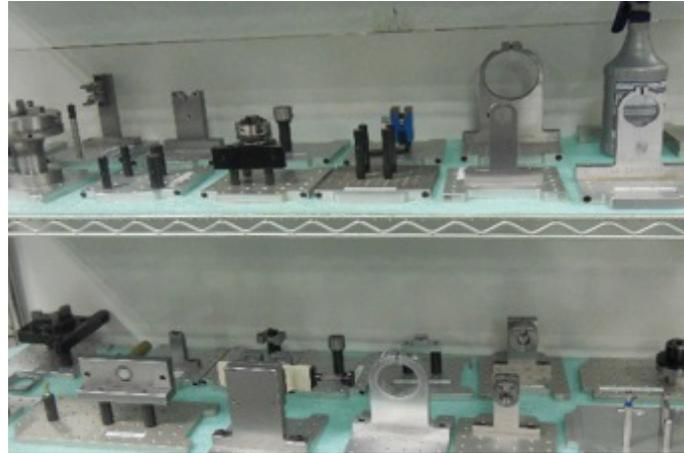
Even if CMM's are upgraded, or added, the Inspection Arsenal™ system can adapt. Simply add a locating rail on the new machines, and fixtures can be moved from one machine to another. Fixture plates and work holding also work on or in conjunction with existing plates.
